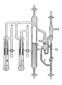
of water through B, mercury from D siphons over into R through the small tube H at the top of F, and seals B once more. The cycle is then repeated. The figure shows the positions of the mercury levels at a certain stage during the up-stroke of the "piston."
